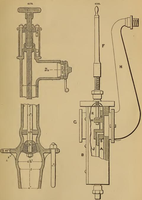
J, discharge-pipe; n, valve-rod; G m, supply-pipe. The valve O is operated by means of the screw stem, which admits the water, while a cavity on the lower edge opens a communication between the discharge and waste pipes. See AIR-CHAMBER. CROWBAR. DRAINAGE. ENGINES, VARIETIES OF. PUMPS AND PUMPING ENGINES.
